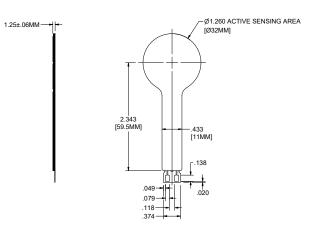
Made of a tough silicone rubber, EAP Sensors can withstand the harshest environments from heat, cold, and shock to dust, vibration and moisture. The resolution, responsiveness and sensitivity are exceptional. The flexible sensors can take accurate measurements and readings while being stretched or compressed for millions of cycles.
